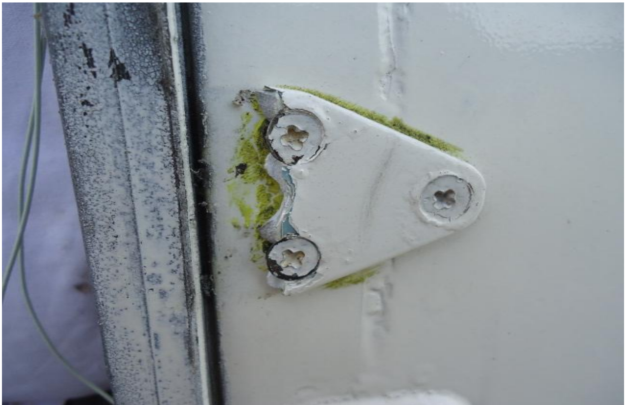
3. Flap door locking plates(upper & lower) were sheared off.
